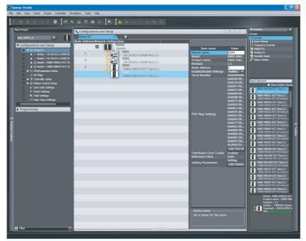
In this example, digital I/O slaves are set to node addresses 1 and 2 and Servo Drives are set to node addresses 3 and 4.
