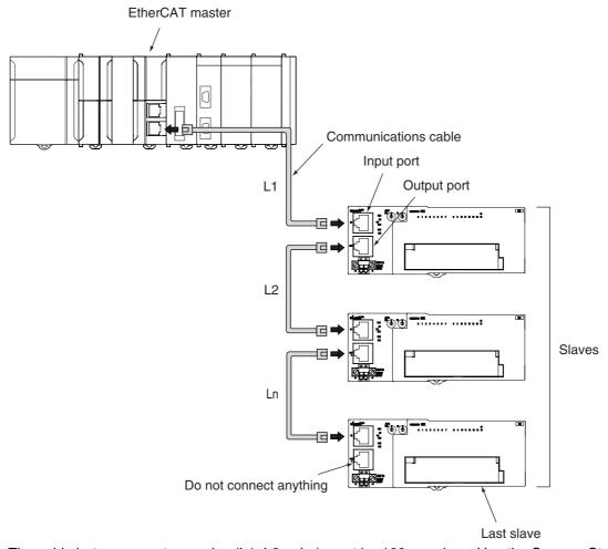
The cable between any two nodes (L1, L2 ... Ln) must be 100 m or less. Use the Sysmac Studio to confirm if communications are possible for the total cable length. Firmly connect the communications cable connector until it clicks into place.
