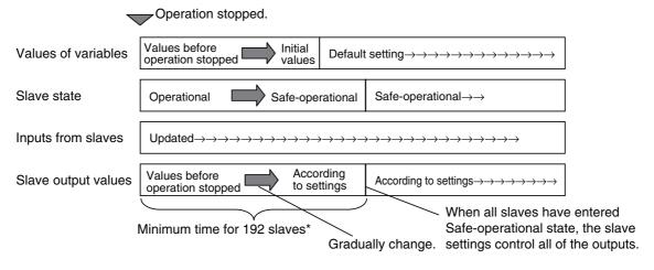
\* If there are 192 slaves connected, the maximum time required for all outputs to be controlled by the slave settings (i.e., the time to enter Safe-operational state) is the communications cycle multiplied by 20 plus the slave Safeoperational state transition time (10 ms max. or OMRON slaves).
