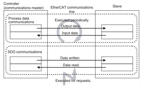
The EtherCAT port built into the NJ-series CPU Unit uses process data communications for commands to refresh I/O data in a fixed control period, including I/O data for EtherCAT slaves, and position control data for Servomotors. It uses SDO communications for commands to read and write data, such as for parameter transfers, at specified times.
