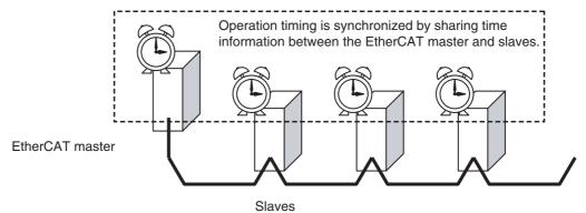
All slaves that support a distributed clock (synchronized slaves) are synchronized with the reference clock. In this EtherCAT system, the closest slave on the network to the EtherCAT master of all the slaves with a reference clock provides the reference clock. The EtherCAT master and slaves automatically access this reference clock.
